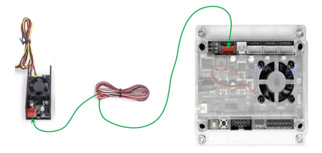
Note: Powering on the machine and connecting the USB Cable can cause the laser module to fire for a short minute. So make sure to have a scrap stock under the laser beam, and also wear your safety glasses before turning the machine on.
